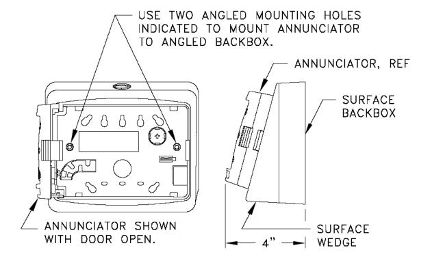
The annunciator surface backbox and wedge can also be fitted to a standard single gang, gangable or 4 'square electrical boxes.
