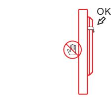
Please use the handle during installation or handling. Please don't touch LCD or other parts, which is a direct reason for device damages, faults or personal injuries.
