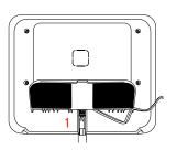
With a small phillips screwdriver, screw in the locking screw from the bottom of the panel to secure it to the table stand.
