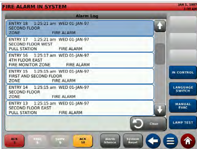
Figure 11: Alarm History Log
