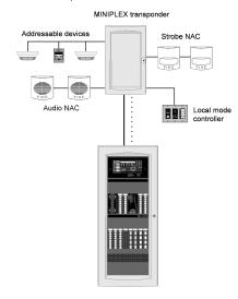
Figure 1: Typical 4100ES MINIPLEX System One-Line Drawing
