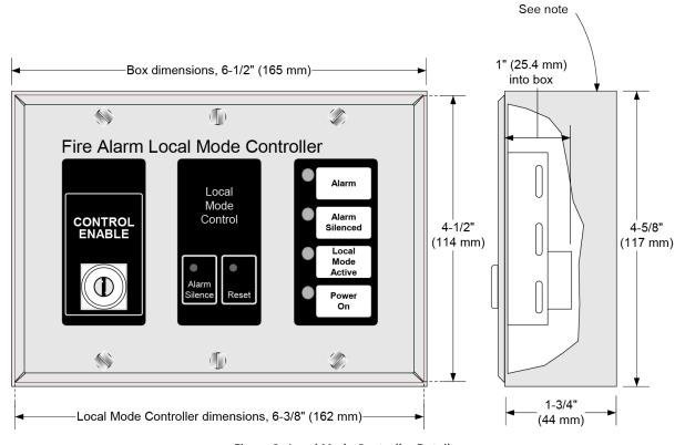
Figure 3: Local Mode Controller Detail
